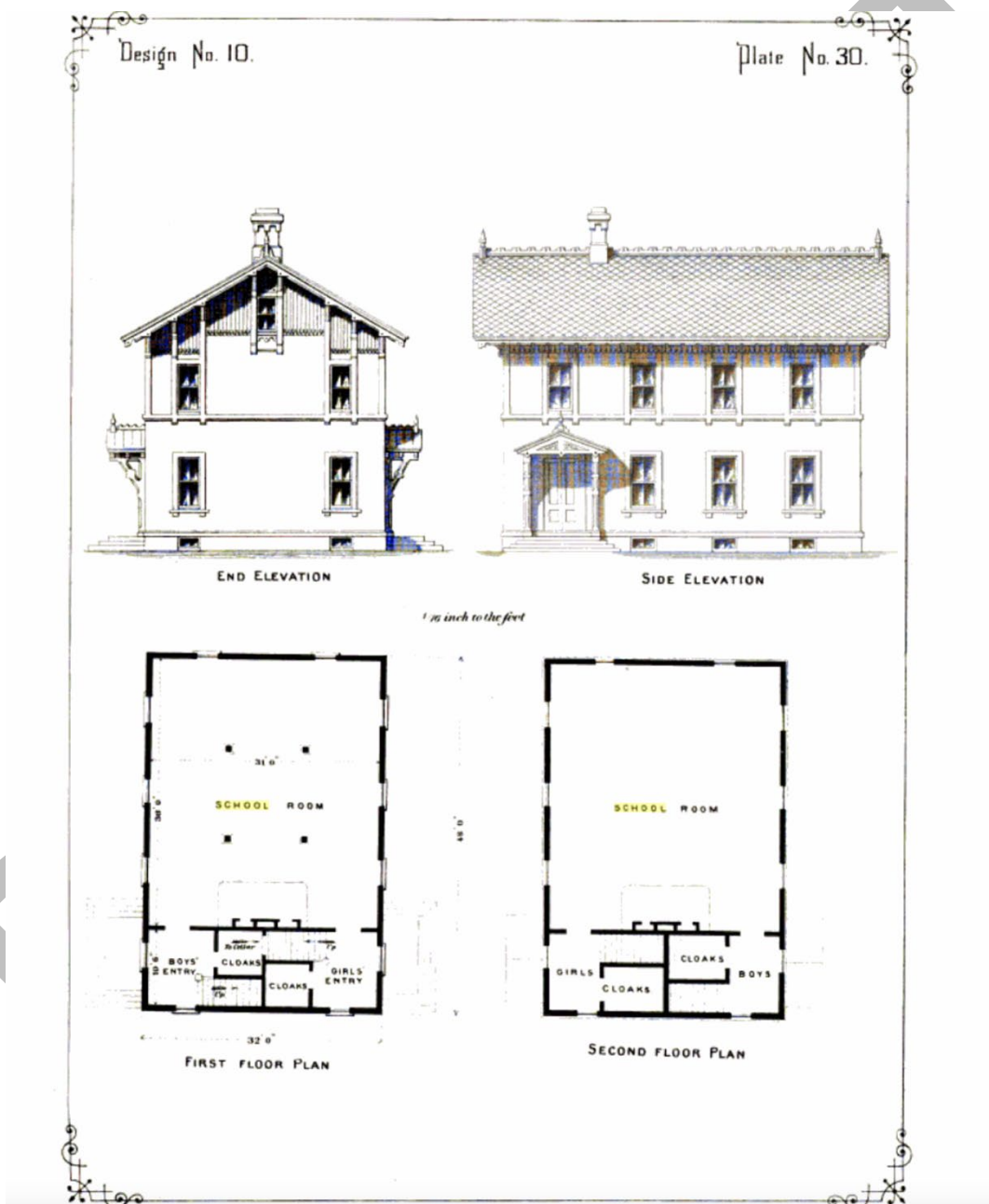
Figure 2. Plan for a model, two-story, two-room schoolhouse. Source: Samuel F. Eveleth, School House Architecture , 1870. Although slightly larger and differing in its entry details and style, this building shares many similarities with Mount Pleasant School and clearly illustrates the influence of the schoolhouse pattern book literature.
